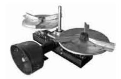
The fertilizer contained in the hopper goes through the dispenser and, due to gravity, falls on the distributor – spreader system.
