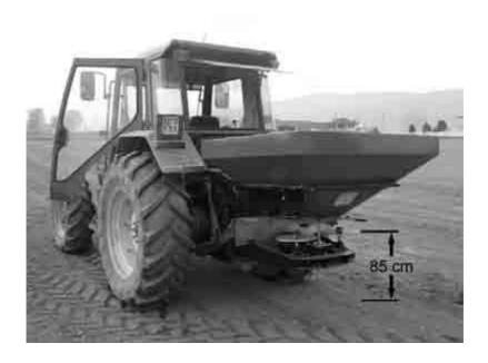
85 cm between the ground level and the distribution disk height
