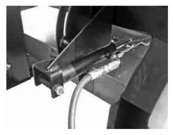
The amplitude of the dispenser opening is manually, adjusted with a lever whose position is fixed on a knob.
